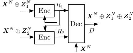
**Fig. 4:** Lossy Interactive Binary sum of two binary sources with presence of a side information
