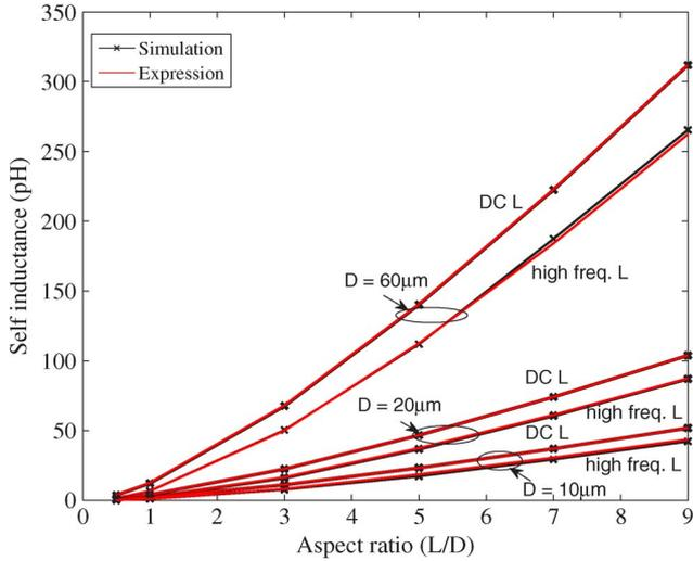
Fig. 5. Self-inductance  $L_{11}$  of a cylindrical 3-D via.
