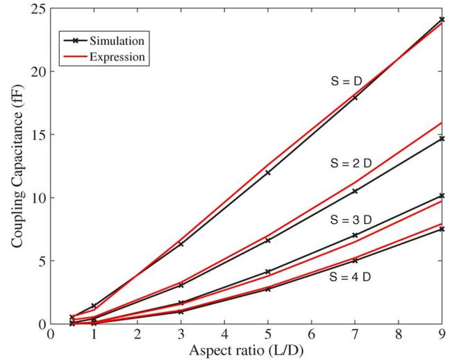
Fig. 9. Coupling capacitance between two 3-D vias over a ground plane ( $D = 20 \mu\text{m}$ ).
