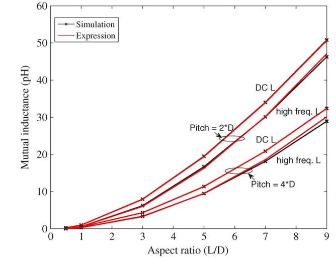
Fig. 6. Mutual inductance  $L_{21}$  for a 20  $\mu\text{m}$  diameter cylindrical 3-D via.
