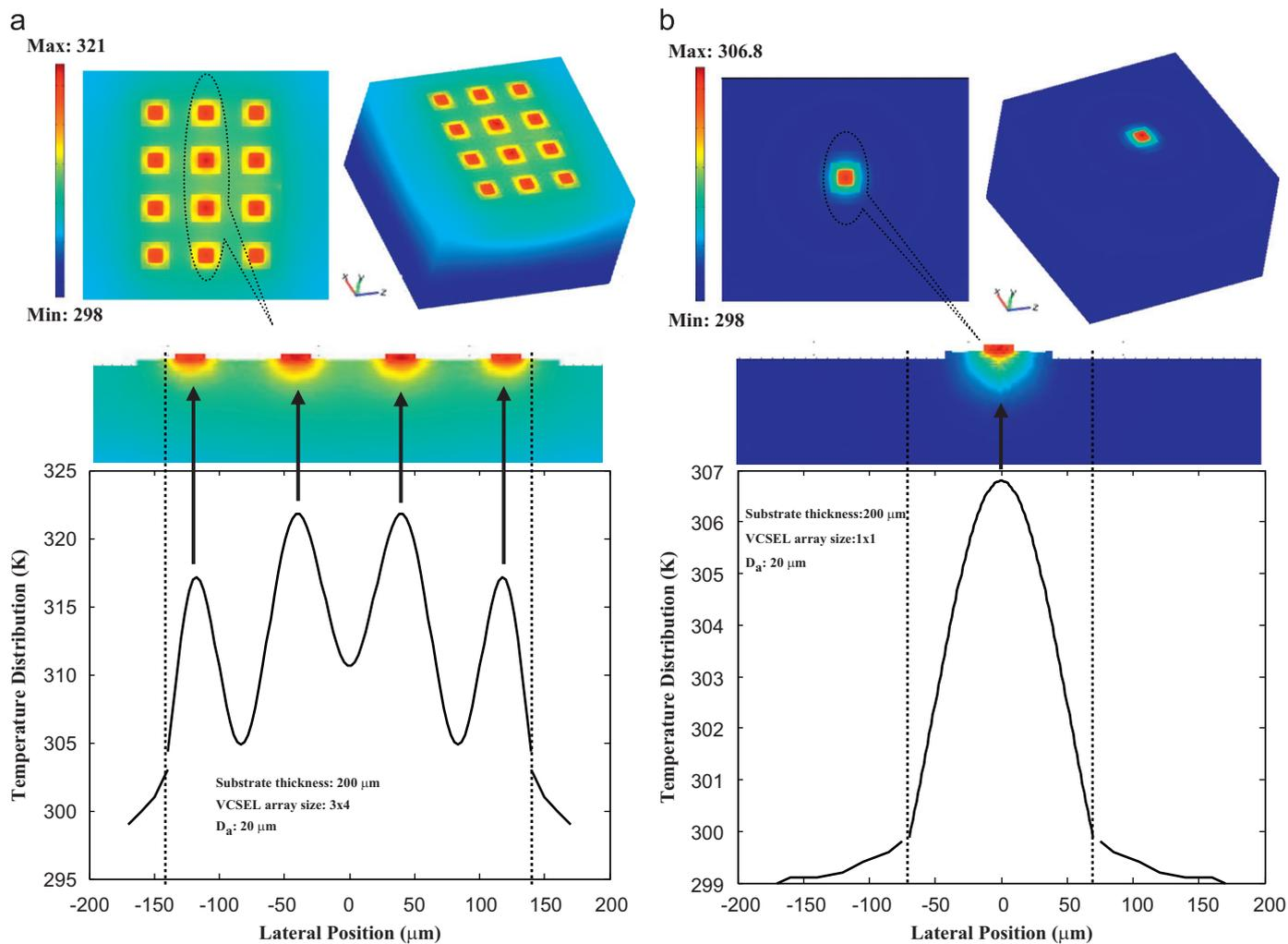
Fig. 2. Heat flux and temperature distribution in lateral direction for (a)  $3 \times 4$  VCSEL array and (b)  $1 \times 1$  VCSEL array.
