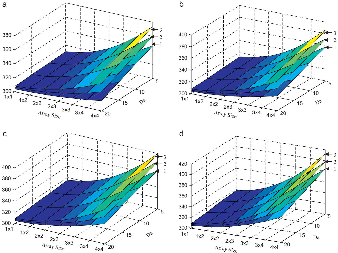
Fig. 3. Maximum internal temperature for several  $D_a$ , VCSEL array sizes, and current densities, (a)  $J=666 \text{ A/cm}^2$ , (b)  $J=800 \text{ A/cm}^2$ , (c)  $J=1000 \text{ A/cm}^2$  and (d)  $J=1200 \text{ A/cm}^2$  1:  $100 \mu\text{m}$  substrate thickness; 2:  $200 \mu\text{m}$  substrate thickness; 3:  $300 \mu\text{m}$  substrate thickness.
