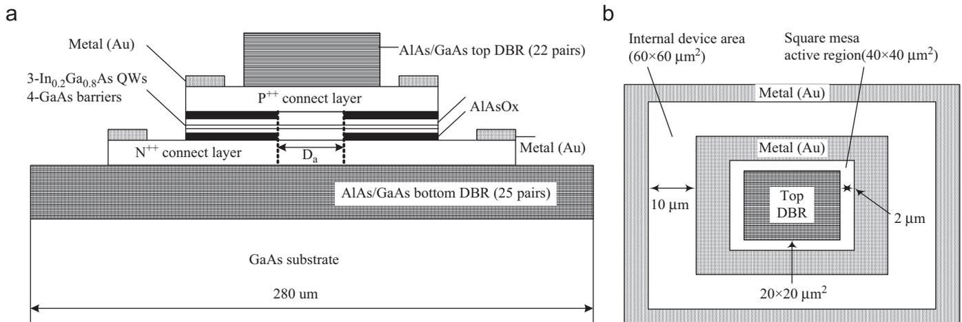
Fig. 1. Schematic diagram of VCSEL structure: (a) side view and (b) top view.
