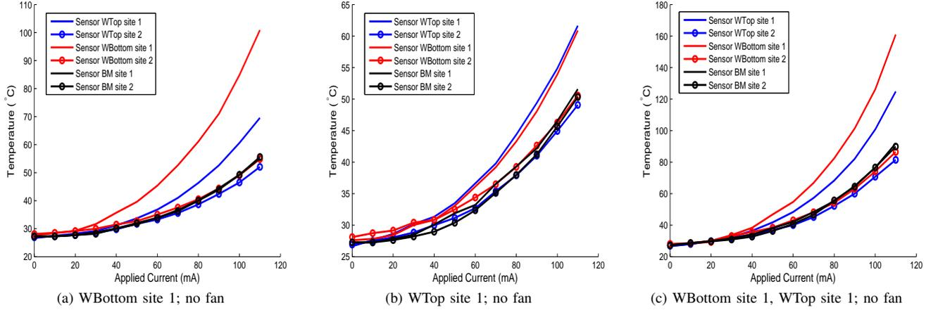
Fig. 3: Experimental results for the different test conditions. Each label describes the device plane, site location of the heater, and whether active cooling is applied.
