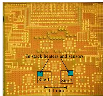
Fig. 2: Microphotograph of the test circuit depicting the back metal pattern with an overlay indicating the location of the on-chip thermal test sites.
