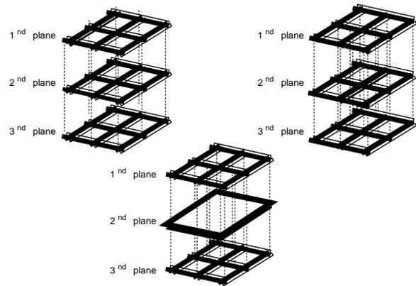
Fig. 3 Three 3-D power distribution networks within the test circuit, (a) TSVs only on the periphery, (b) 50% higher TSV density as compared to (a), and (c) dedicated plane for power and ground distribution.
